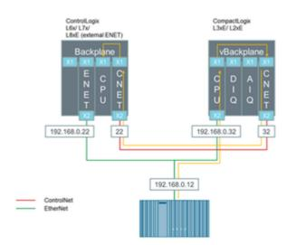
The yellow line in the above image represents the communication path (route parameters). In the communication path, the red marked sections always contain a network specific address. The blue marked part identifies the backplane or the interface to be used. It is not important that the backplane is physically existing or virtual. The green part identifies the slot number of the next bridge module (next hop) or the destination module.
